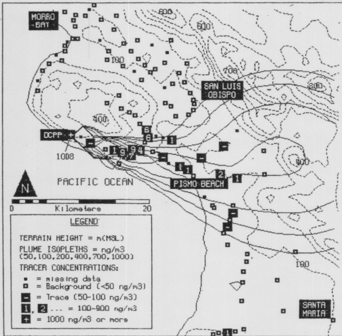
Figure 5. Comparison of MIDAS and PGEMS model output with SF6 gas tracer data for 9/09/86 at 1500 PDT
