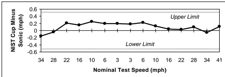
Unlike an anemometer, the sensing elements of the ultrasonic wind sensor are oriented differently depending on wind direction. This presented a possibility that a wind speed bias might exist based on the direction of the wind. To address this concern, TVA rotated the sensor in  $5^\circ$  increments and measured wind speeds in each position. The resulting samples (12 five-second values) are summarized in Figure 2. No irregularities are evident for any directions.
