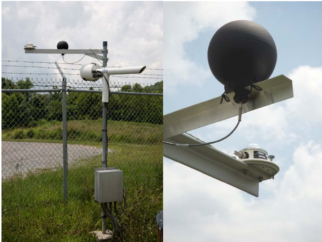
Figure 2. Globe temperature installation at one of the Y-12 NSC meteorological towers
