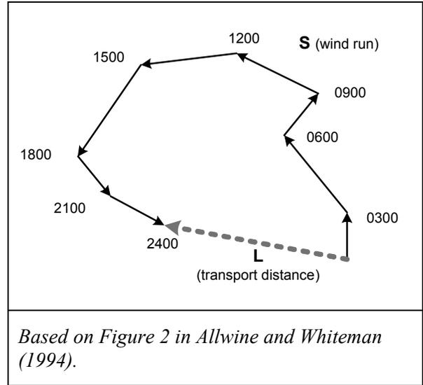
**Figure 1: Illustration of wind run (S) and transport distance (L).**
